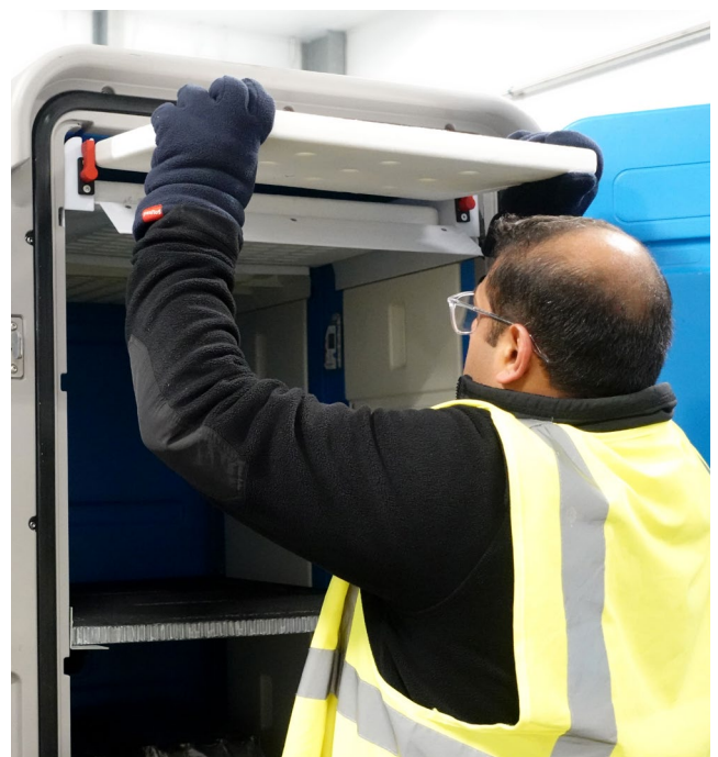
Photo: A CoolRun pod being loaded with PCM, Hubli; UK - 2024
