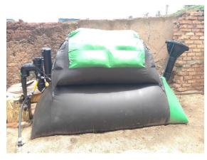
Figure 2 Anaerobic digester by HomeBiogas, Source: BBOXX.
